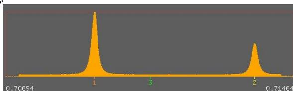
**Figure 2.** X-ray spectrum of the Mo diffractometer at Utrecht University
