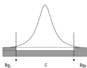
**Figure 4.** Background-Peak-Background method for the determination of  $I$  and  $\sigma$ .
