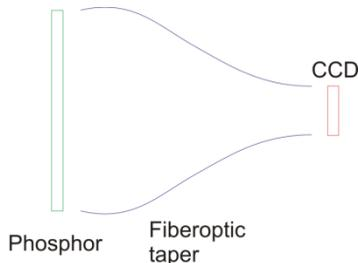
**Figure 5.** Schematic drawing of a CCD detector.
