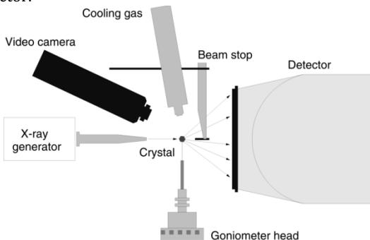
**Figure 1.** Setup of a single crystal diffractometer
