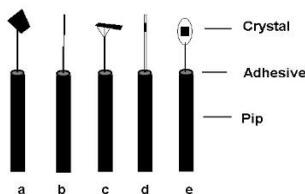
**Some methods for mounting crystals: a) on a glass fibre; b) on a "two-stage" fibre; c) on a fibre topped with several short lengths of glass wool; d) within a capillary tube; e) in a solvent loop.**
